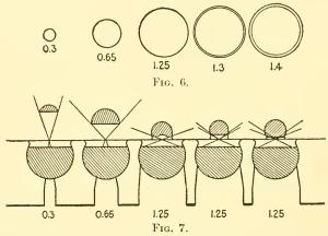
Fig. 6. This shows the objective aperture circles and the condenser aperture circles seen on the back of objectives of the five named apertures, with a condenser cone of a maximum aperture of 1.25. The radii are made proportional to the apertures.
