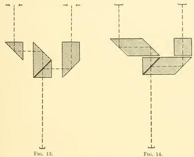
Fig. 13.—Diagram of the prisms in the original Jentzsch monobjective binocular. The double line indicates the semireflecting surface of silver or platinum. The interocular distance is altered by shifting out or in the two outer prisms, which are attached to the eyepieces. This of course increases or decreases the optical tube length. Note that there are two reflections on each side.
